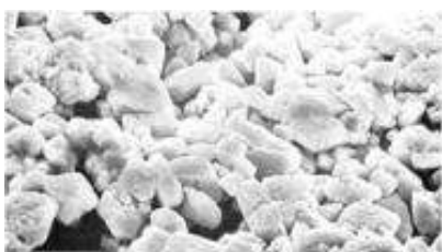
Figure 10-1: Crystalline formation on NiCd cell.
