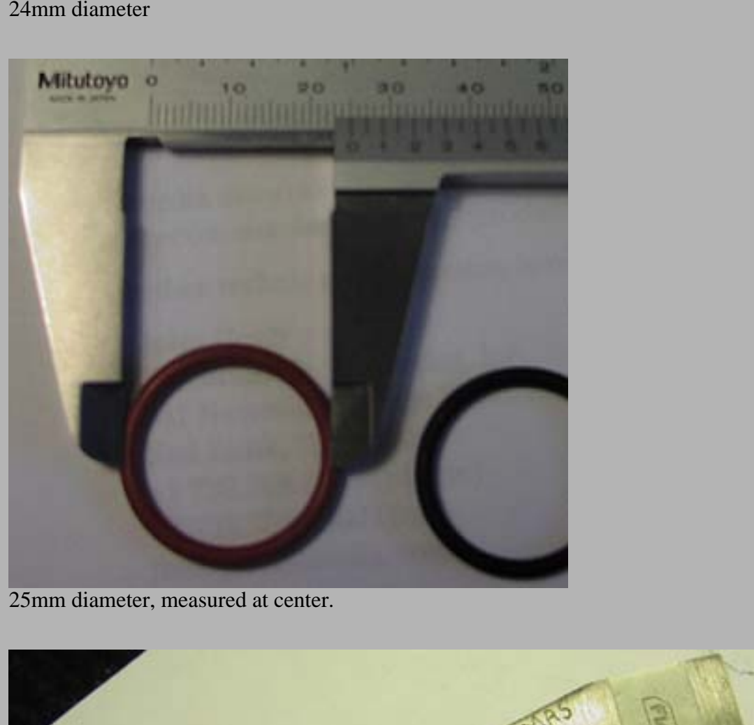
The black type is a bit more strong, and not so elastic; compared to the red one.
